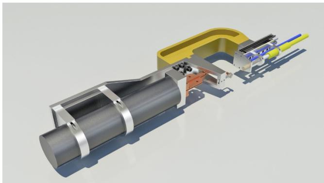
**The joining gun bonds metal and plastic in seconds and can be mounted on a robot arm in place of a spot welding gun, for example.**
